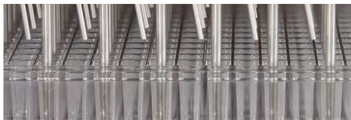
384-well plate washing: Dispense and aspirate tip positioning.
